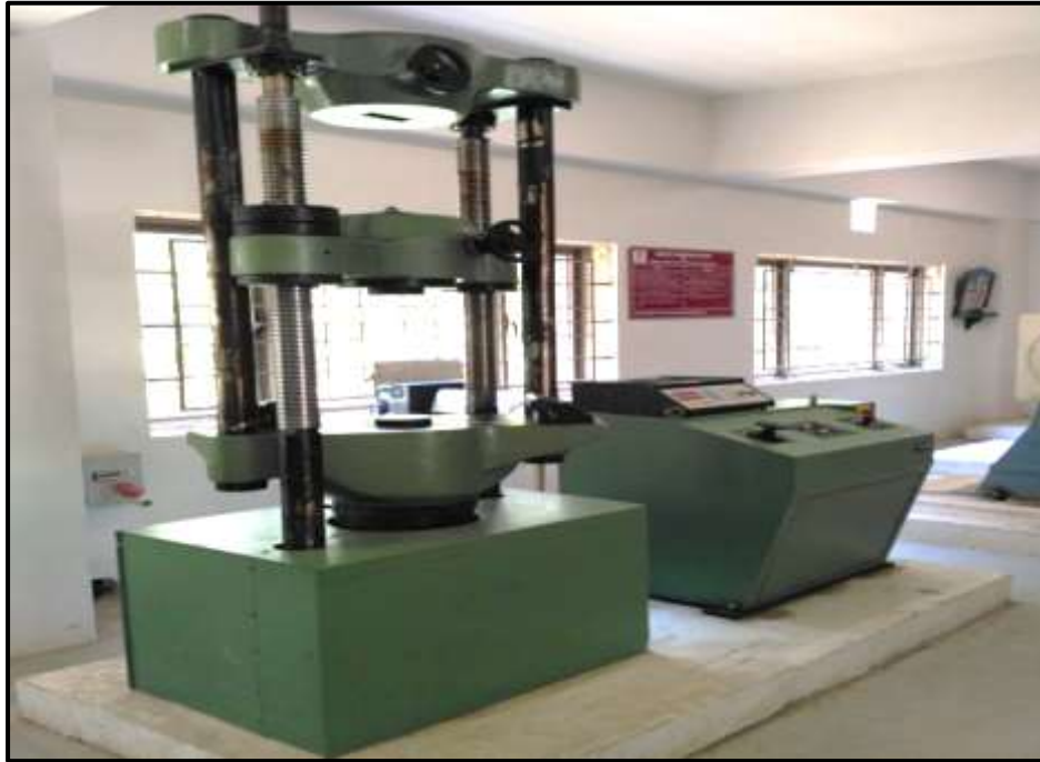
Electronic Universal Testing Machine in Mechanics and Materials Testing Lab
