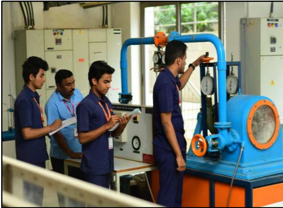
Pelton Wheel Turbine test rig in Fluid Mechanics and Fluid Machinery-Lab
