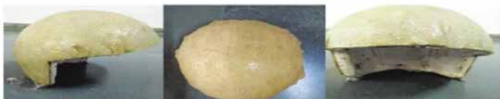
HARD AND HEARTY | These helmets made from pineapple leaves are stiffer than commercially available gear
