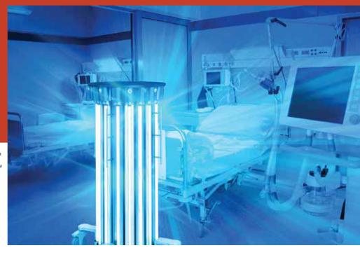
The use of commercial proprietary equipment for UV-C radiation of the environment entails a significant cost to acquire the equipment and maintain it, because it is a proprietary technology. Most of the available equipment use low-pressure mercury lamps to produce UV-C radiation. These lamps can be acquired separately and used in the disinfection device we have created.
